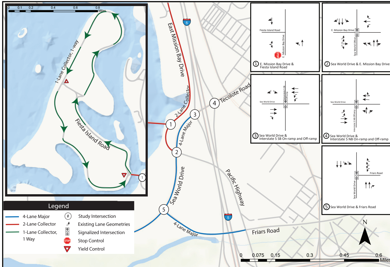
Figure 2-16 Existing Intersection Geometry and Functional Classifications
