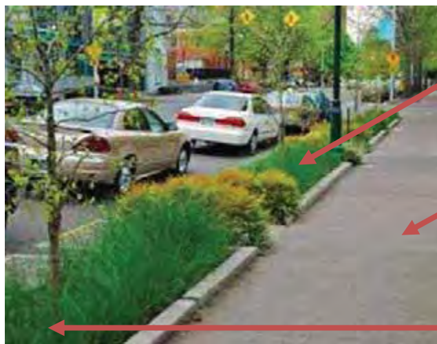
Figure 1: Illustration of Sample Structural BMP: Green Streets
