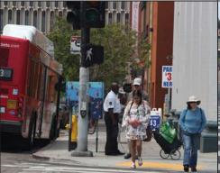
**Lead Pedestrian Intervals** provide pedestrians a 3-7 second head start when entering an intersection, reinforcing their right-of-way over turning vehicles.
