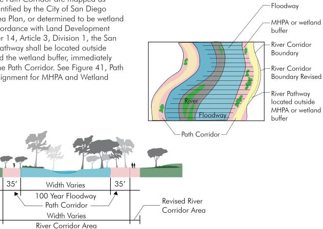
Figure 41: Path Corridor Realignment for MHPA and Wetland Buffer
