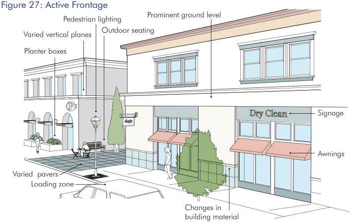
**DG-39 Limitations on Blank Walls.** Minimize the amount of the linear frontage on the first story street-facing wall that may consist of blank walls. Where blank walls are unavoidable, reduce the impact by:
