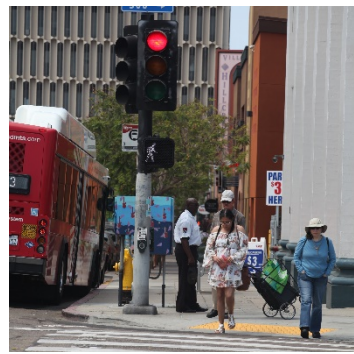
4. Lead Pedestrian Intervals provide pedestrians a 3-7 second head start when entering an intersection, reinforcing their right-of-way over turning vehicles.
