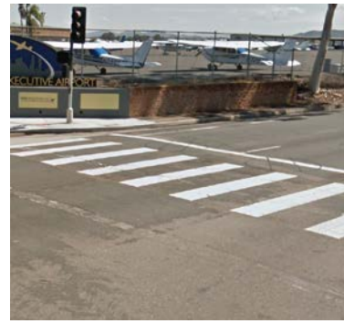
1. Continental Crosswalks Improve crosswalk visibility and are known to improve driver yielding compliance.
