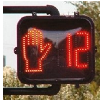
2. Pedestrian Countdown Signals provide pedestrians with a clear indication of how many seconds remain to safely cross.
