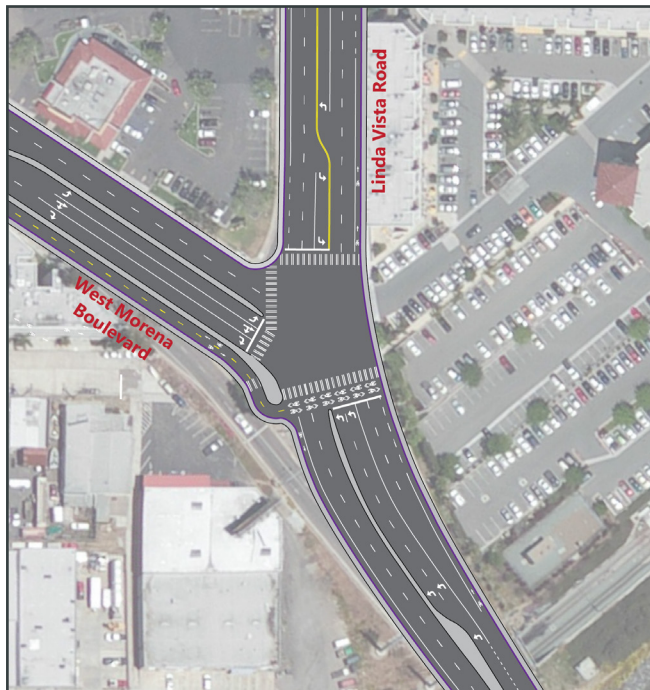
Figure 3-8 - Proposed Intersection Conceptual Design for Improvement 6
