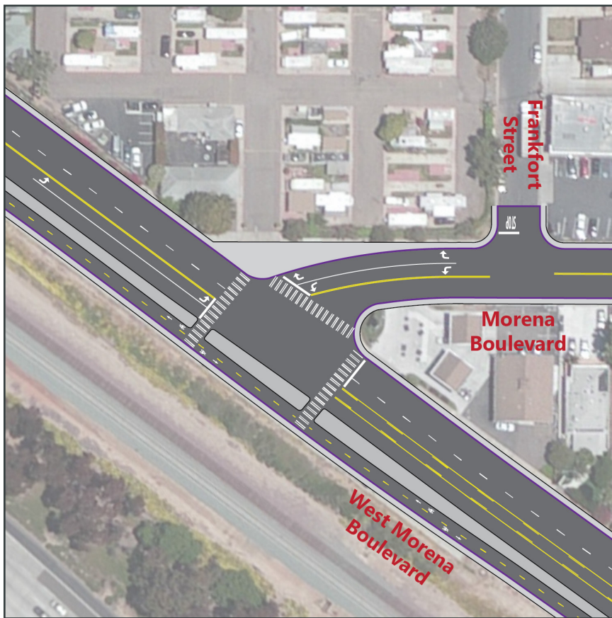
Figure 3-4 - Proposed Intersection Conceptual Design for Improvement 2
