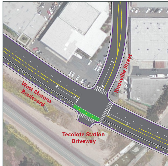
Figure 3-5 - Proposed Intersection Conceptual Design for Improvement 3
