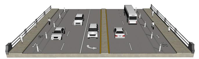
Conceptual design of enhanced Class II bicycle facility along Clairemont Drive at the I-5 Overpass bridge.
