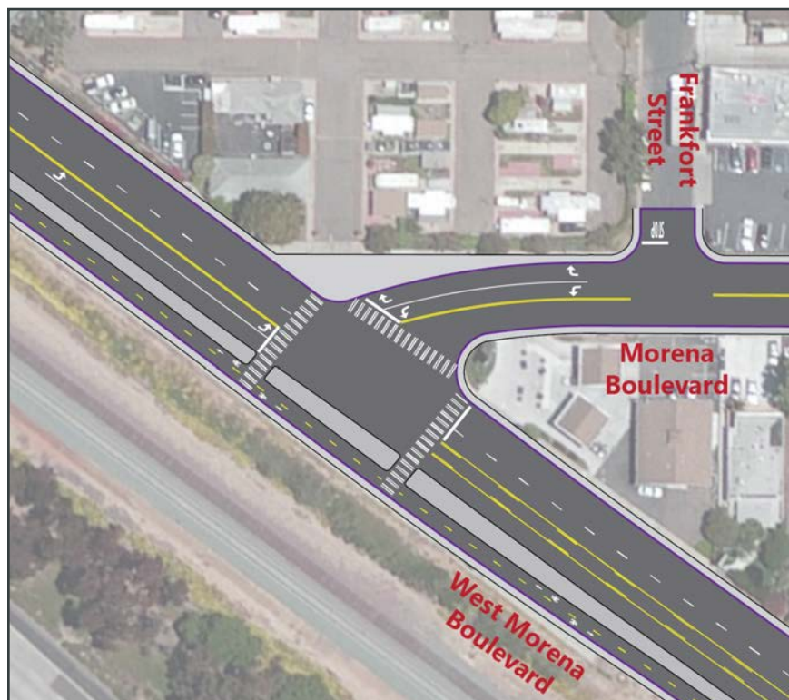
Figure 3-4 - Proposed Intersection Conceptual Design for Improvement 2
