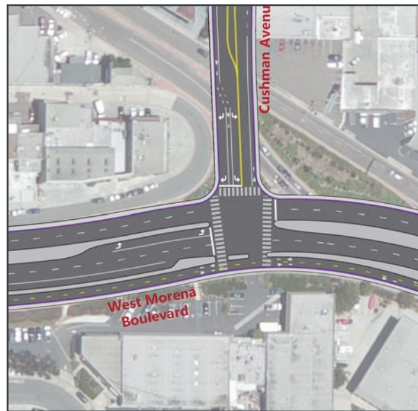
Figure 3-9 - Proposed Intersection Conceptual Design for Improvement 7
