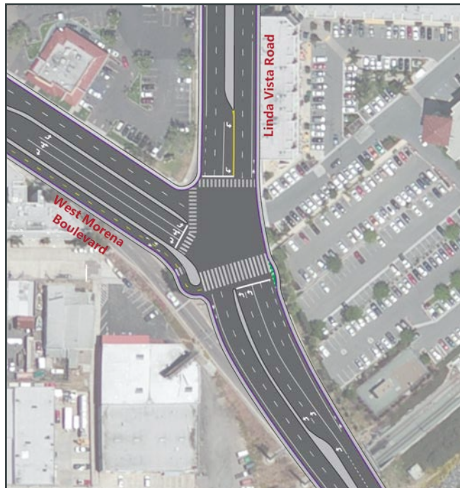
Figure 3-8 - Proposed Intersection Conceptual Design for Improvement 6
