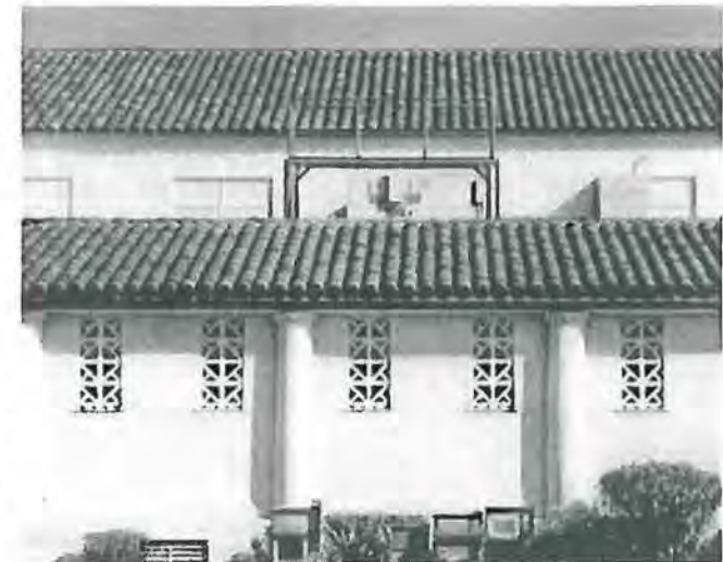
These new mechanical units greatly distract from the architecture of the historic district. Mechanical units have been installed where they are visible from the public realm and are not acceptable. The design and placement of newspaper stands should be considered as to not distract from the historic setting. Photograph courtesy of Architect Milford Wayne Donaldson, FAIA, January 11, 2000.
