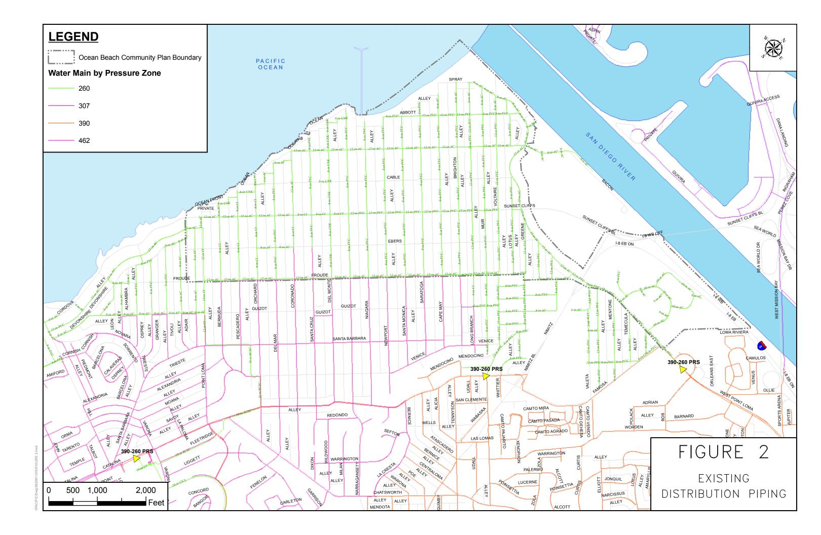
The three pressure reducing stations which feed the Point Loma 260 Pressure Zone provide redundancy so that if ever one station was out of service, water delivery to the Point Loma 260 Pressure Zone would not be interrupted. Redundancy ensures that public health and safety are protected in that water quality and quantity are maintained to the public and fire fighting capability is always assured.
