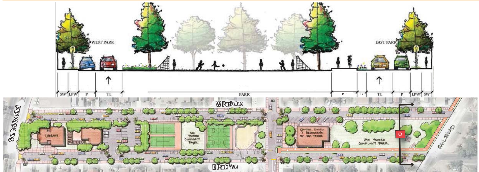
Example streetscape in plan view, featuring connected sidewalks, landscaping, crosswalks, and Cycle Track.
