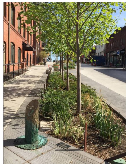
Bio-retention and/or bio-filtration features will be incorporated into the Pacific Highway streetscape to help address storm-related flooding and downstream water quality.
