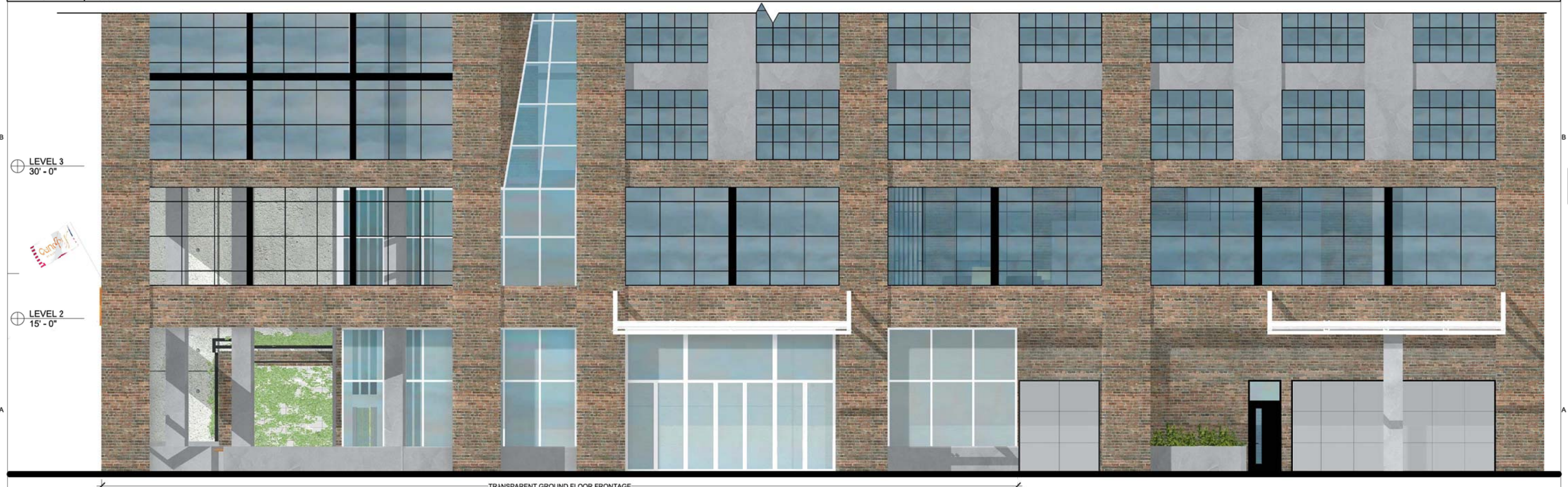
A1 EAST ENLARGED ELEVATION 3/16" = 1'-0"
