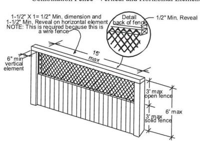
Combination Fence--Vertical and Horizontal Elements
