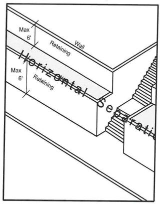
Horizontal separation <u>distance shall be</u> <u>greater than or</u> equal to <u>the</u> height of the upper wall
