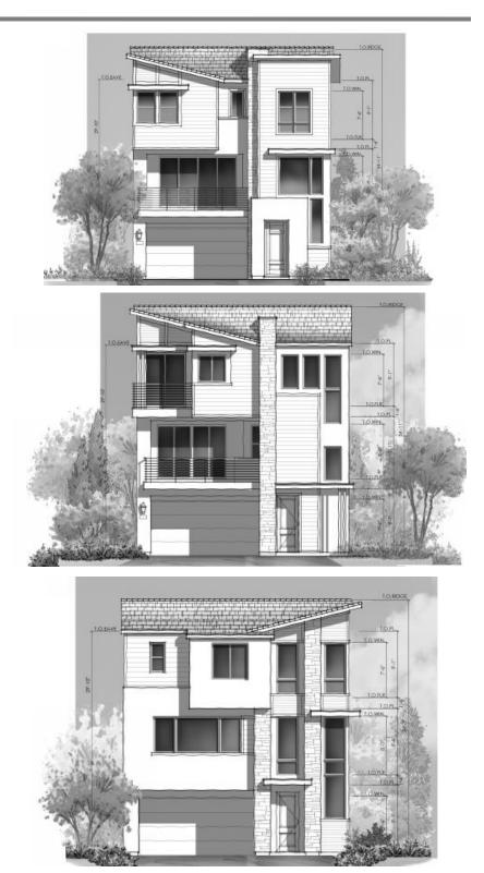
Figure 7 – Typical Contemporary California Elevations
