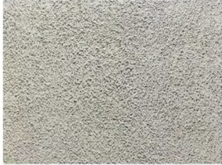
(1) Stucco 20/30 Sand Finish To match paint specs
