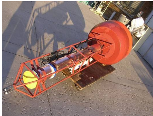
Figure 2. Drawing and a photograph of the Scripps-designed coastal buoy system for measuring stratification and currents at the Point Loma Ocean Outfall.
