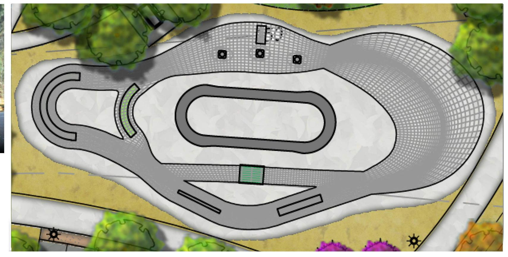
BICYCLE PLAYGROUND - CONCRETE PUMP TRACK CENTER RING WITH OUTER CONCRETE AGILITY COURSE RING - POTENTIAL COLORED CONCRETE
