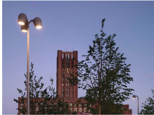
Photo 6.7: Multiple luminaires can be attached to a single pole for greater lighting emphasis.
