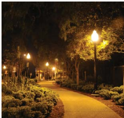
Photo 3.24: Lighted Pathways. Consistently spaced pedestrian scale luminaires.
