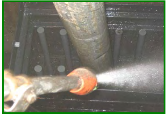
Spray Down and Clean Cartridge Filter Housing
