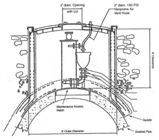
Air relief assembly and maintenance hatch.
