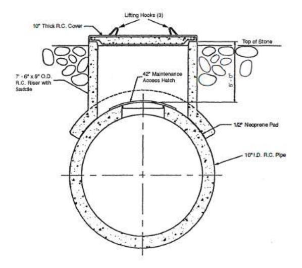
Maintenance access hatch and riser.
