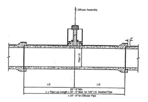
Diffuser assembly on the SBOO Diffuser Legs.
