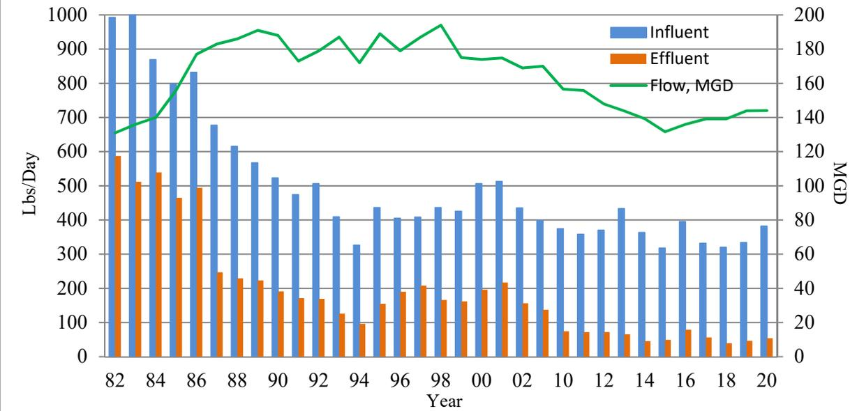
Figure 1.2-2 Long-term trends of Pt Loma plant flows and influent and effluent loadings of potentially toxic heavy metal pollutants are shown above.
