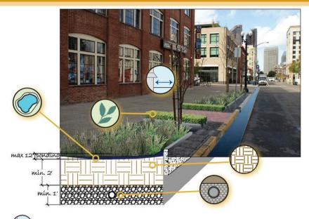
**Existing Buildings:** Assess building effect (runoff, solar shadow) on the site. Bioretention systems must be set away from building foundations at least 10 feet.
